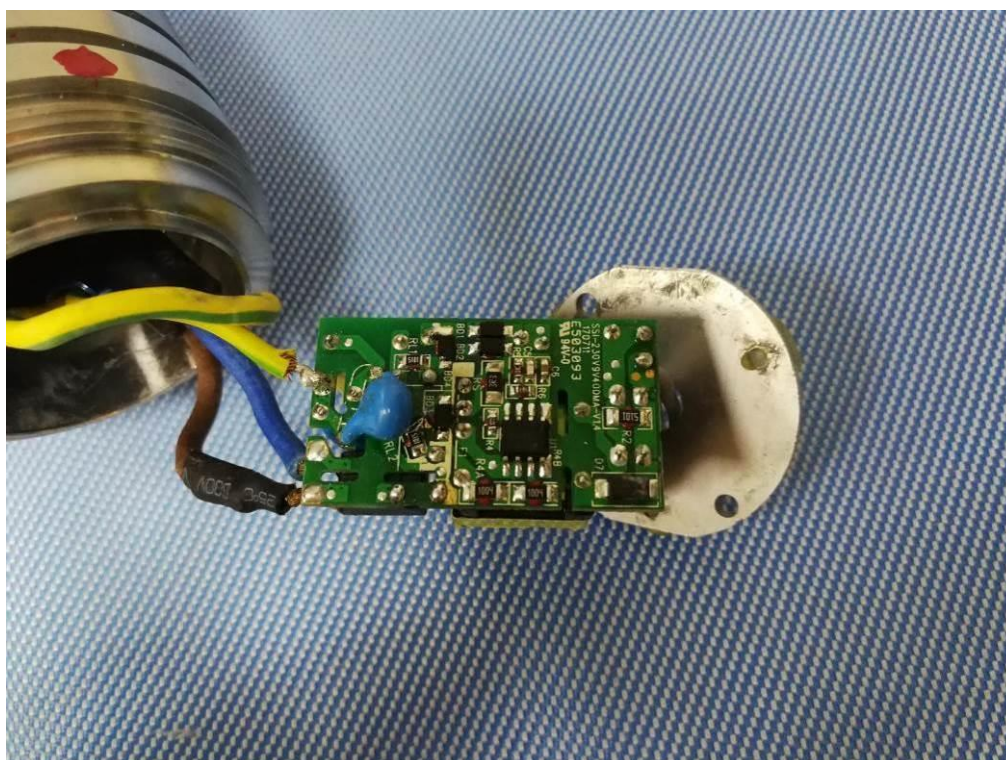
Picture 10. The wire conductor is inserted into a hole in a printed board, bent and soldered, the hole having a diameter slightly greater than the conductor
